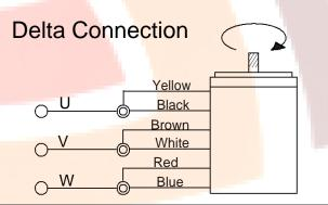
To change the direction, interchange any two wires between U, V & W
