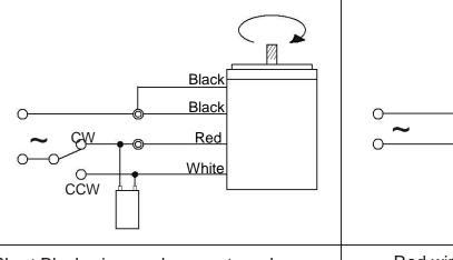
Short Black wires and connect as shown to rotate the motor in clockwise direction
