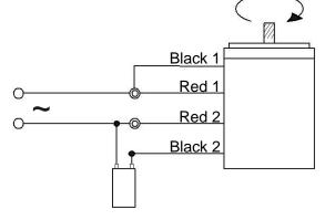
Red wires are for running winding & Black wires are for starting winding
